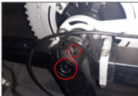
Crank screws must be tightened, with no space between crank and support
