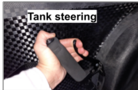
C3.3 The lever / levers must function gradually. After released, it / they should go back. The stationary brake have to be handled with ease.
