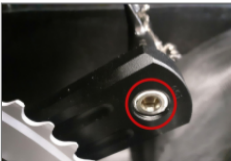
Crank screws must be tightened, with no space between crank and support
