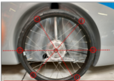
C5.3 Wheel must be correctly centered into the wheel arch. Verify on the horizontal line, several pairs of points.
