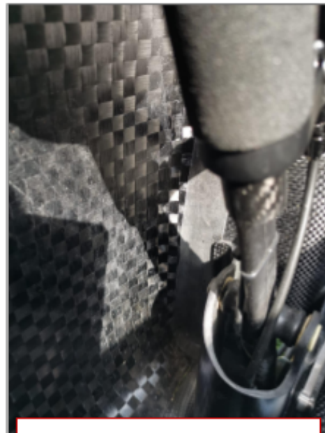
C4.2b Tank-steering: has no play and moves easily
