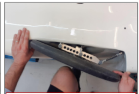
C5.4 Pull to the sides to check play in the suspension or rod bar ends
