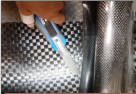
C8.1 Check proper gluing with a cutter
