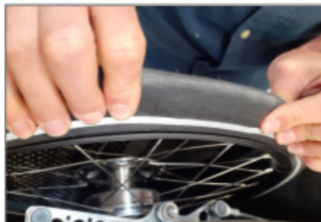
B4.4 The inner tube must not be jammed
