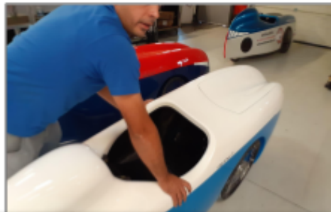
C3.2 With the stationary brake on, check both sides. Raise the vehicle on each part pushing down on the wheel to see if the brake keeps resistance.
