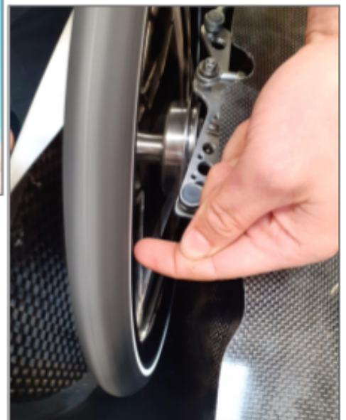
C5.7 Must be straight. Tolerance: 1 mm
