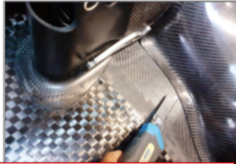
C8.1 Check proper gluing with a cutter
