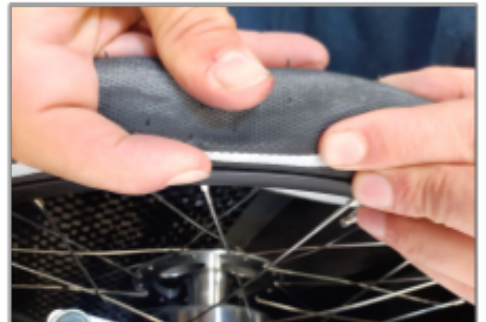
B4.3 The jacket must not have transport damage
