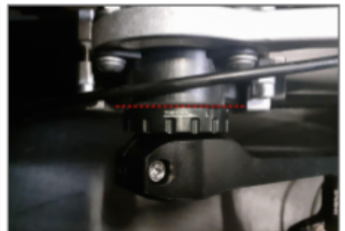
Crank screws must be tightened, with no space between crank and support
