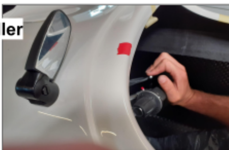
C3.3 The lever / levers must function gradually. After released, it / they should go back. The stationary brake have to be handled with ease.
