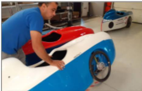
C3.2 With the stationary brake on, check both sides. Raise the vehicle on each part pushing down on the wheel to see if the brake keeps resistance.
