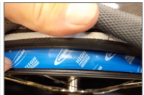
B4.6 Double layer rim tape properly centered
