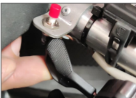
B12.4 Gear shift lever must not touch horn button support
