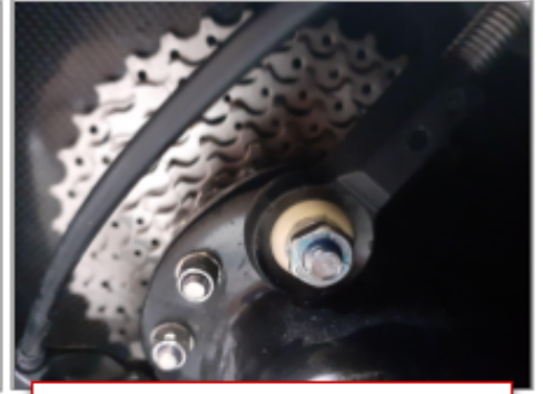
B18.3 The M6 counter nut must be secured with Loctite
