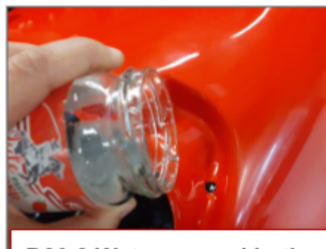
B20.2 Water poured in the drainage hole does not get inside the vehicle
