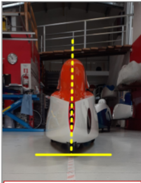
A8.4 With vehicle on wheels, the rear wheel has to be perpendicular to the contact surface
