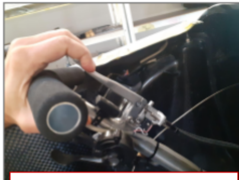
B12.2 The lever must function gradually
