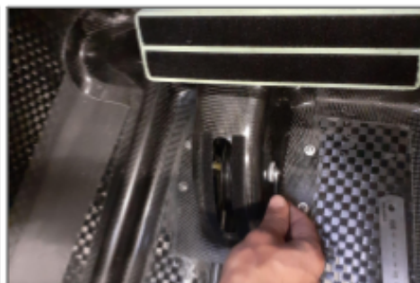
B5.4 The axis must be tightened
