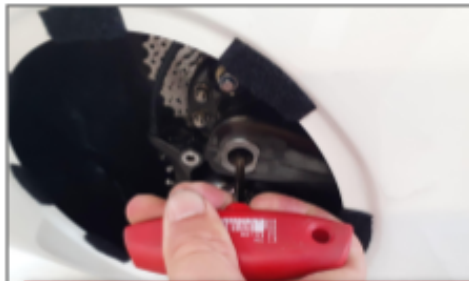
B18.4 The screw of the bearing must be fixed and Loctite present. Bullet label has to be present that was factory checked.
