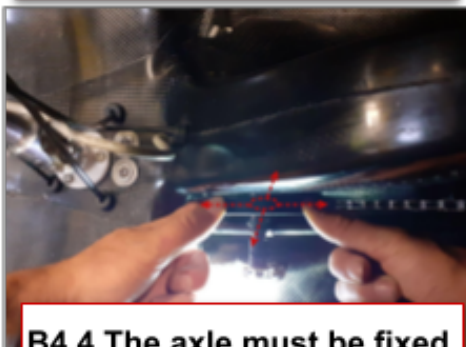
B4.4 The axle must be fixed in the left 8mm hole in the carbon
