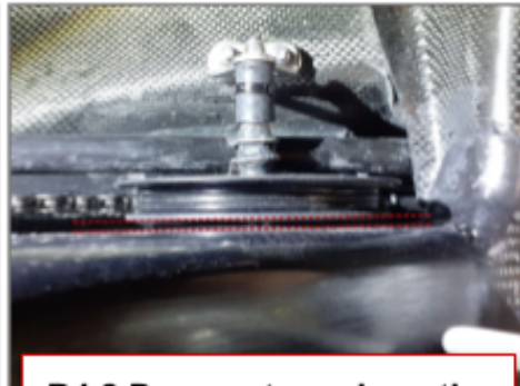
B4.2 Does not scrub on the carbon frame or chain tube
