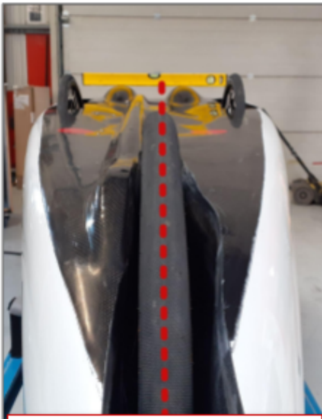
A8.3 The wheel must be vertical, 90° from the bottom body surface
