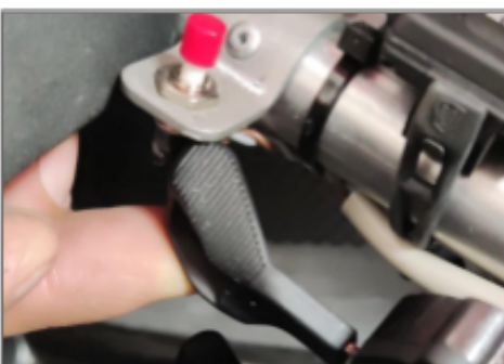
B12.4 Gear shift lever must not touch horn button support
