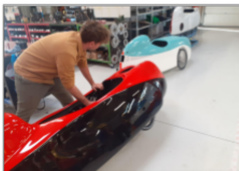
B12.5 Check that breaks work on each side and that they are balanced.
