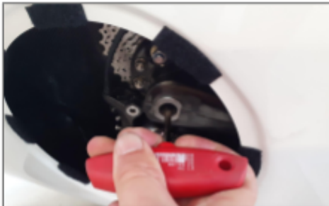
B18.4 The screw of the bearing must be fixed and Loctite present. Bullet label has to be present that was factory checked.
