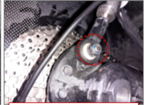
B18.3 The M6 nut must be locknut
