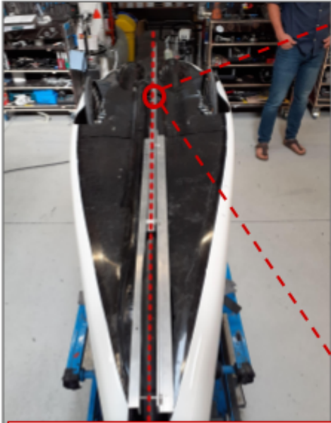
A8.1 The wheel must be aligned with the longitudinal axe and in the center of the wheel arch
