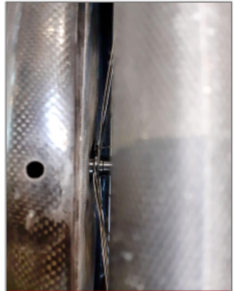
A8.2 The wheel arch must not rub against the spokes or the cassette
