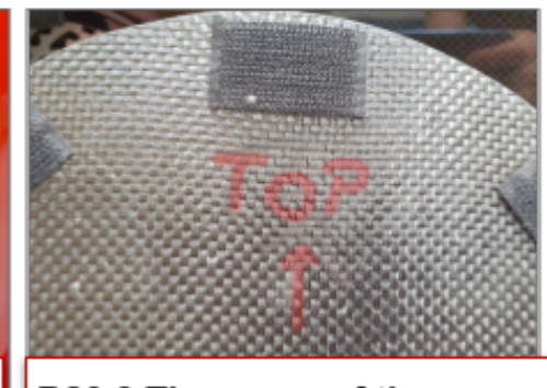
B20.3 The cover of the rear cassette has to be mounted with inside arrow top
