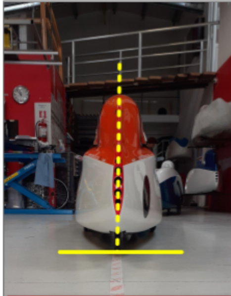
A8.4 With vehicle on wheels, the rear wheel has to be perpendicular to the contact surface
