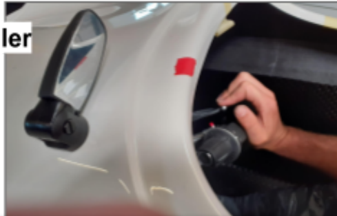
C3.3 The lever / levers must function gradually. After released, it / they should go back. The stationary brake have to be handled with ease.
