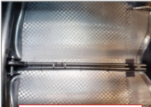
C7.1 Chain tubes have to be tied with clamps
