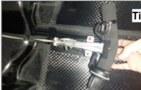
C3.3 The lever / levers must function gradually. After released, it / they should go back. The stationary brake have to be handled with ease.
