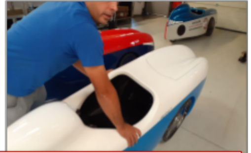
C3.2 With the stationary brake on, check both sides. Raise the vehicle on each part pushing down on the wheel to see if the brake keeps resistance.
