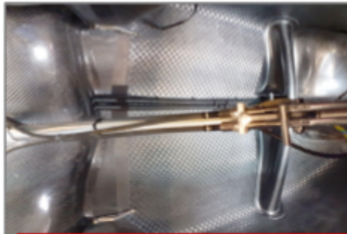
C7.2 Clamps on the steering neat cut to not scratch cyclist's feet.
