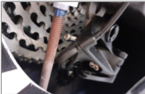
C9.2 The end stops must be set ( safety relevant ).
