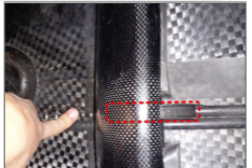
C9.4 The idler should be straight and not rub
