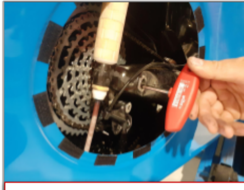
C8.2 The screw of the bearing must be fixed and have Loctite.
