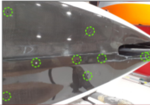
All holes pointed in photos to be present, neat and clean
