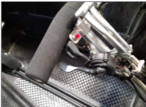
B15.4 Gear shift lever must not touch horn button support or the tiller
