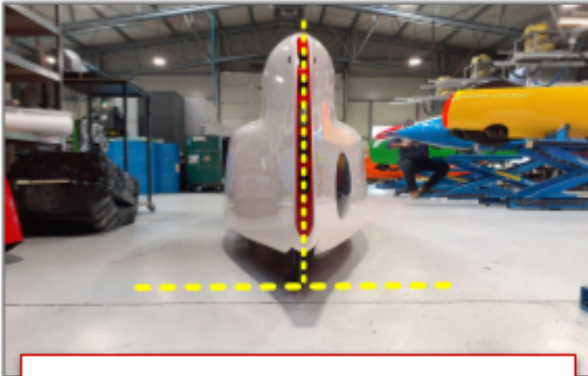
B18.1 The rear wheel must be perfectly vertical.
