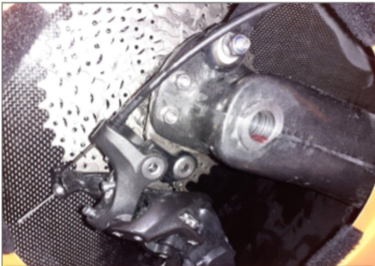
B17.4 Lock nuts, tightened according to: (check with the torque tool) Derailleur bolt: 8Nm Derailleur hanger on Swingarm: 6Nm Shiftcable Rear Derailleur: 8NM (Shimano)/~6Nm (Sram)
