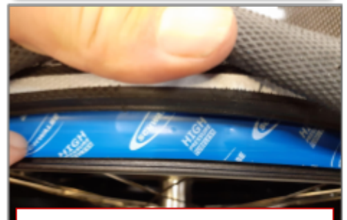
A4.6 Double layer rim tape must be centered Front wheel: 25mm Rear wheel: first layer 19mm, above 21mm.
