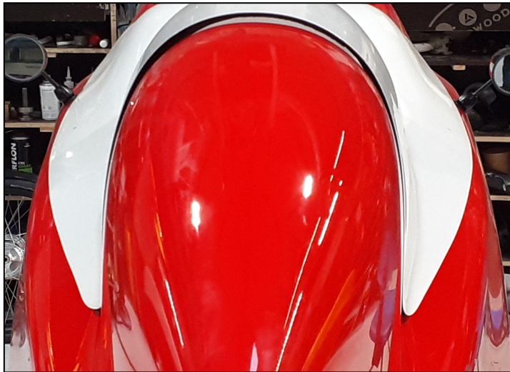
B23.3 Hood is properly aligned and symmetrical
