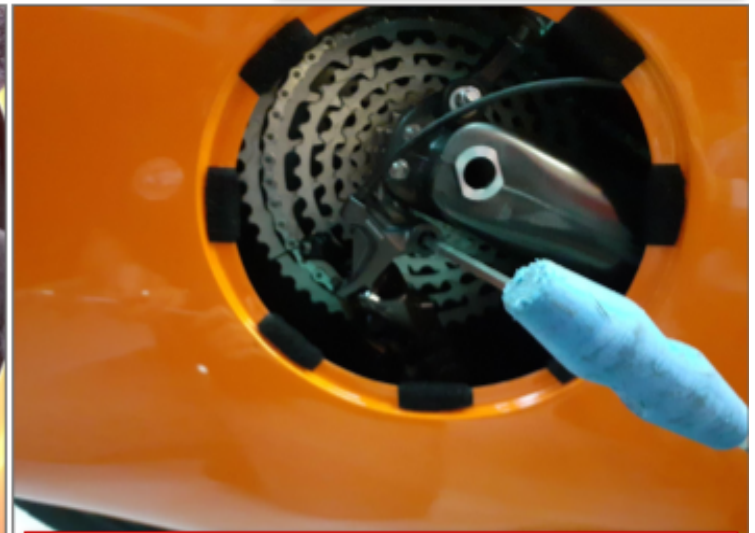
B17.5 Well tightened support screw
