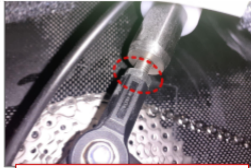
B17.2 Low nut M8 DIN 439 A2 must be present
