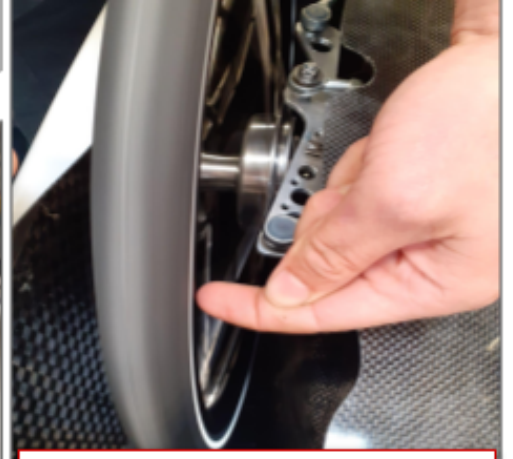
A5.5 The wheels must be straight. Tolerance: 1 mm
