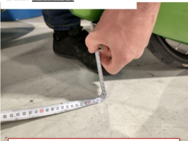
B22.1 Rear distance to ground are between 175 and 180 mm.
