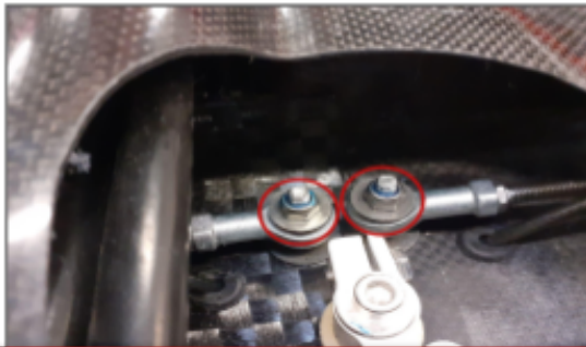
A3.3 Rod ends to be well tightened with locker nuts
