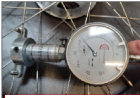
A5.3 Spoke tension must be between 1200 and 1400N
