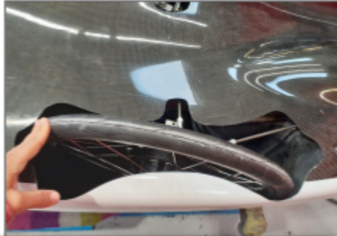
A5.1 The wheels must not touch the cutouts
