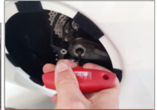
B17.3 The screw of the bearing must be fixed and Loctite present. Bullet label has to be present that was factory checked.
