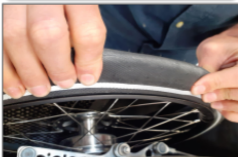
A4.4 The inner tube must not be jammed
