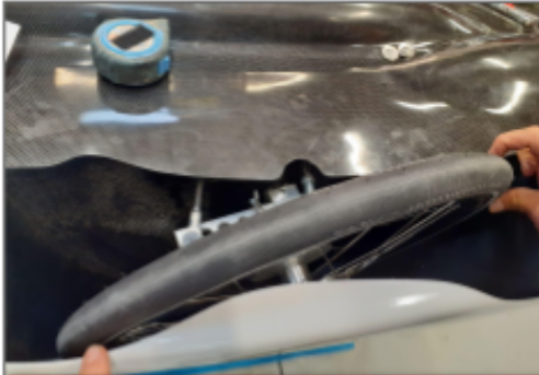
A5.1 The wheels must not touch the cutouts
