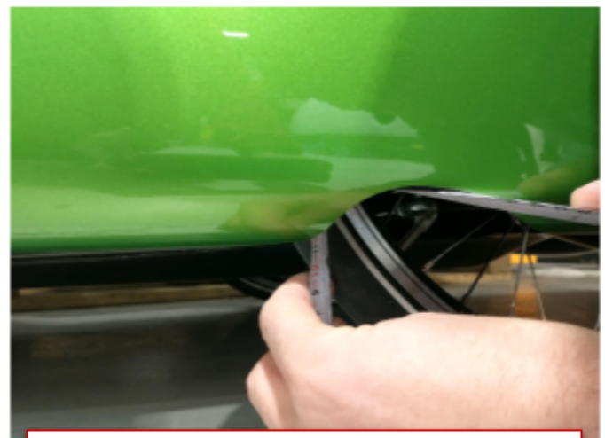
B22.2 Behind front wheels, both distances to ground are between 110 and 115 mm.
