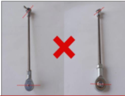
A2.3 All ball joints to be aligned
