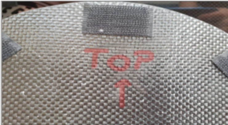
B20.3 Side cover has "Top" mark properly oriented
