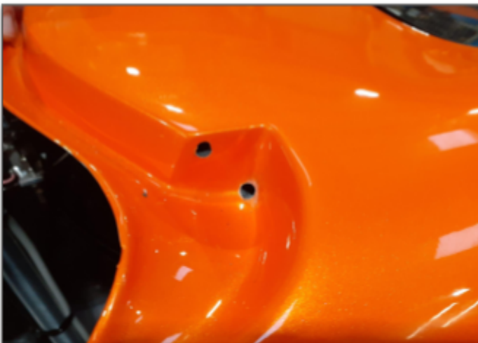
B19.1 Check that poured water in the water drain does not get inside vehicle
