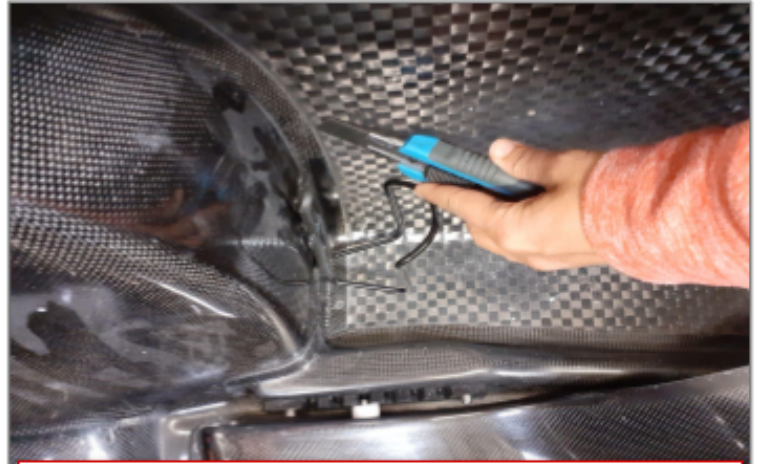
B20.2 Verify gluing with a cutter blade
